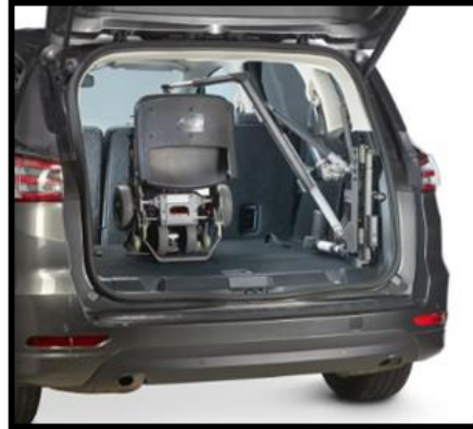
Figure 4 - Trunk Mounted Arm Hoist
