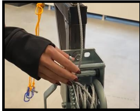
Figure 8 - Ensuring that the Locking Mechanism is in the Lowering Position
