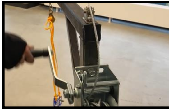
Figure 9 - Clockwise Rotation of the Crank to Lower the Clips
