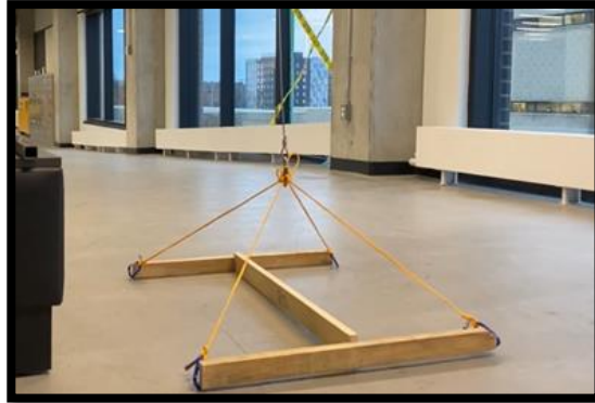
Figure 11 - Walker Slightly Lifted in a Stable Position
