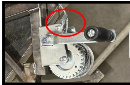
Figure 15 - The Locking Mechanism on the Crank Circled in Red
